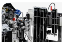
Purification system on "stand- alone" structure
