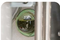
Oil sight glass with autopstop
