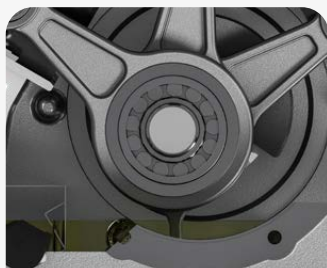
Splash lubrication with conrod pin immersed in oil
