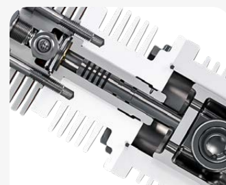
Third stage in tempered steel with 5 piston rings in special cast iron
